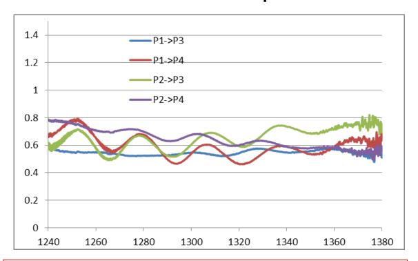
Filter-Based Wideband Coupler with IL Variation of 0.2 dB
